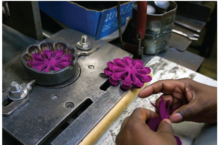
Employee Alex Nelson using the “clicker” or die-cutter machine to stamp out flower shapes in multiple layers (left). Molding three dimensional petals with the hot press (below).
