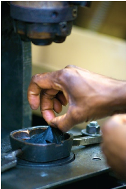
Molding leather in the hot press machine (left). Employee Musa Drammeh shaping flower petals out of white fabric at one of the hot press machines (above).
