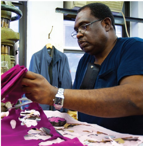
Employee Alex Nelson using the “clicker” or die-cutter machine to stamp out flower shapes in multiple layers (left). Molding three dimensional petals with the hot press (below).
